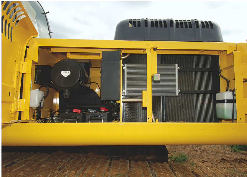
The SK350LC's batteries are easily serviced from ground level, along with the air cleaner. The new side-by-side coolers are smaller than those of the predecessor model and can be individually serviced. The air-conditioning condenser is positioned some 5 inches away from the surface of the other coolers so as not to impede airflow.
