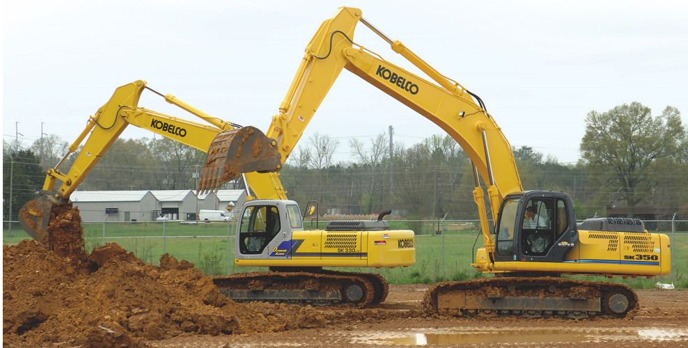
The test machines, both low-hour units that were checked for pertinent specifications before the comparisons, used standard digging arms (10 feet 10 inches) and identical heavy-duty, 48-inch-wide, 2-cubic-yard buckets.
