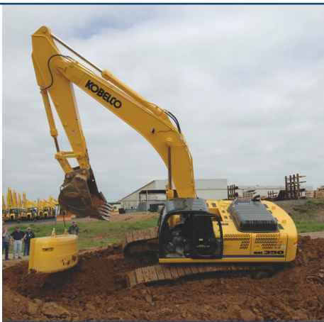
The SK350LC remained impressively flat-footed during the swing-torque test.
