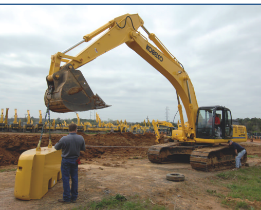
The nearly 20,000-pound test weight (an excavator counterweight) provided a reasonable challenge for the test machines.
