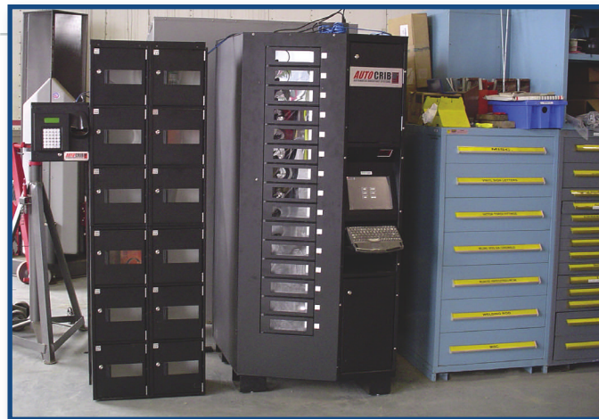
The parts vending machine at Alyeska Pipeline Service Co. sits in the middle of the shop floor for easy access by technicians. The machine is equipped with a scanner, keyboard and screen.
