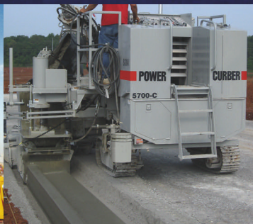
Power Curber 5700-C Curb and gutter, sidewalks
